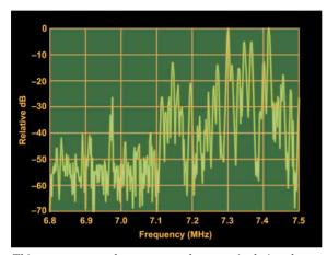
This spectrum analyzer screen shows typical signal levels on frequencies between 6 800 and 7 500 kHz in the eastern United States during the early evening. There are many amateur signals between 7 000 and 7 300 kHz, but the band between 7 100 and 7 300 kHz is dominated by European broadcasting signals.
